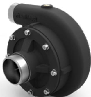
The VFT\_2SP is a compact, efficient and reliable 2-stage centrifugal pump. The body and impellers are made of anti-corrosive aluminum. The axis and other components are made of stainless steel. Includes a high-quality mechanical seal specifically designed for the Vallfirest pumps.
